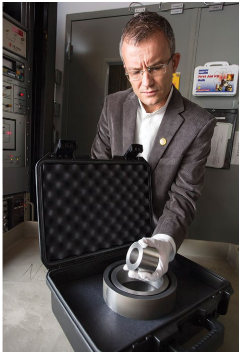
Assistant Professor Alex Glaser displays a device known as the “British Test Object,” which simulates the materials used in a nuclear warhead and is used for testing methods of verifying the authenticity of the weapons.
